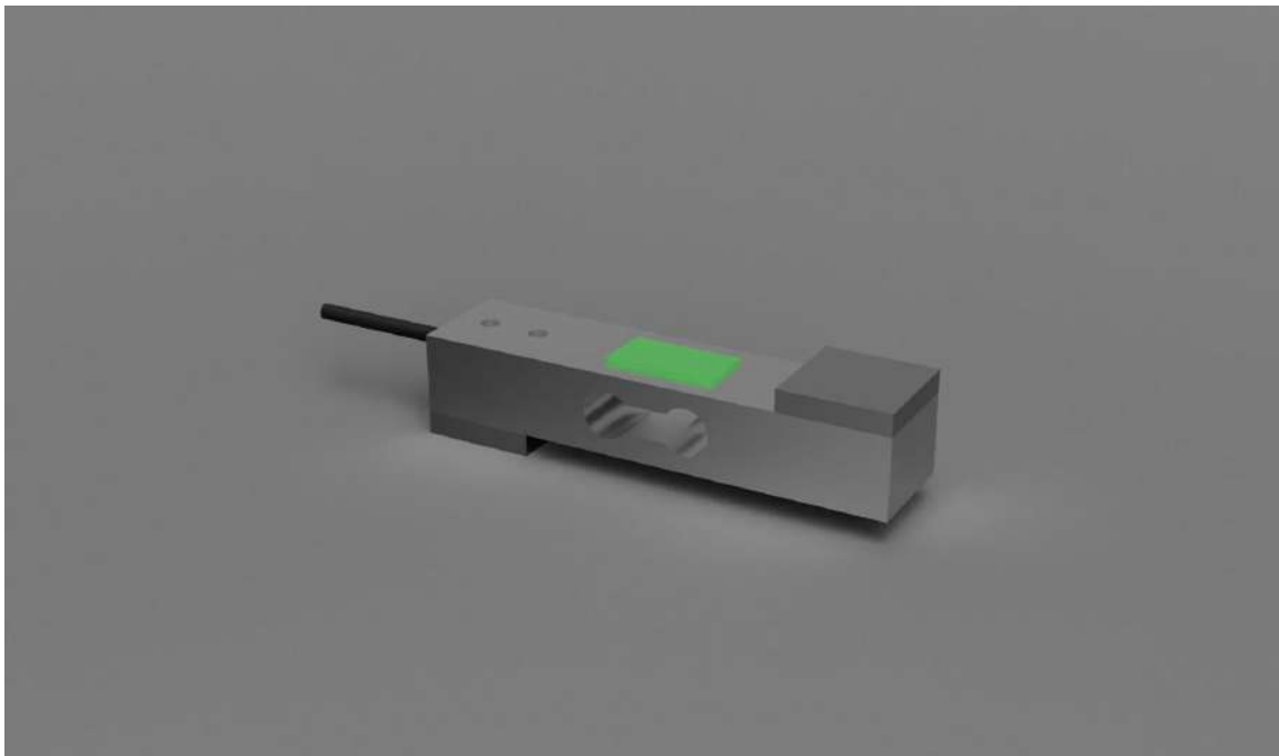
Bar load cell: the dumbbell hole concentrates bending strain under the potted strain gauges; the 4-wire cable runs to the HX711
