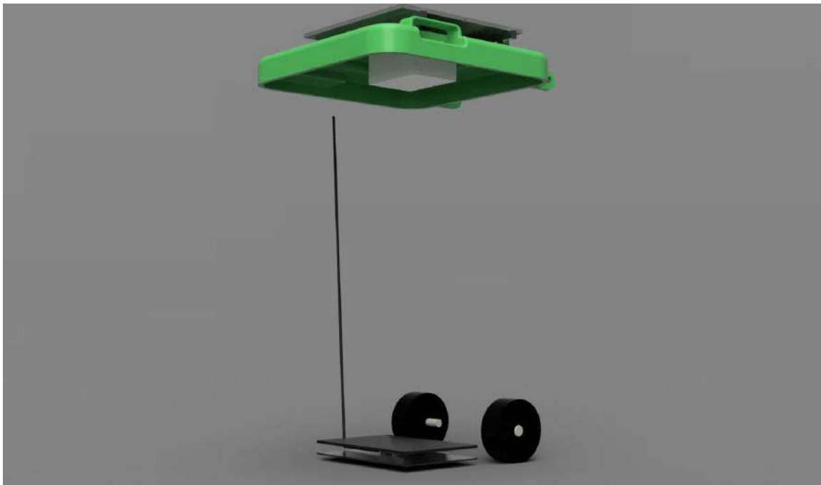
Internal layout with the bin walls hidden: electronics under the lid, weighing platform on the floor, load-cell cable up the side wall
